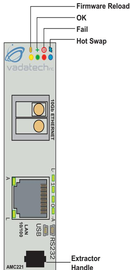
FIGURE 2. AMC221 Front Panel
