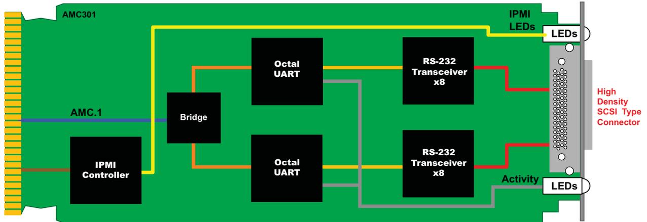
FIGURE 1. AMC301 Functional Block Diagram
