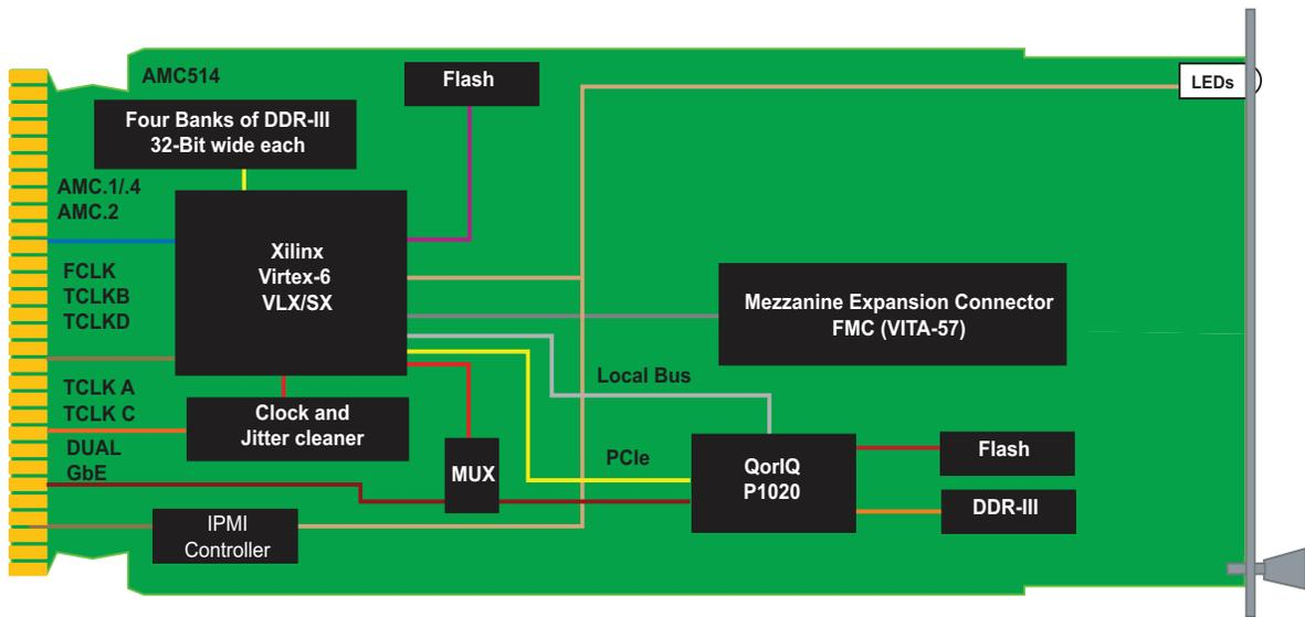
FIGURE 1. AMC514 Functional Block Diagram
