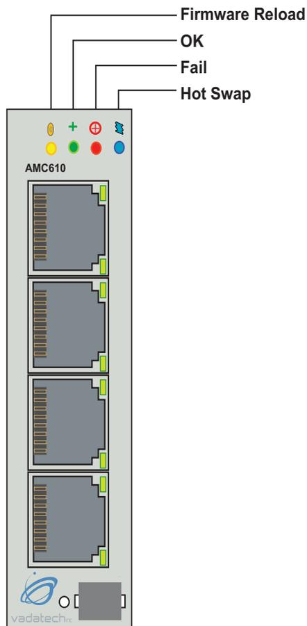
FIGURE 2. AMC610 Front Panel
