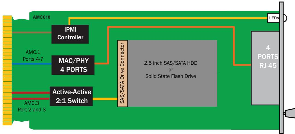
FIGURE 1. AMC610 Functional Block Diagram
