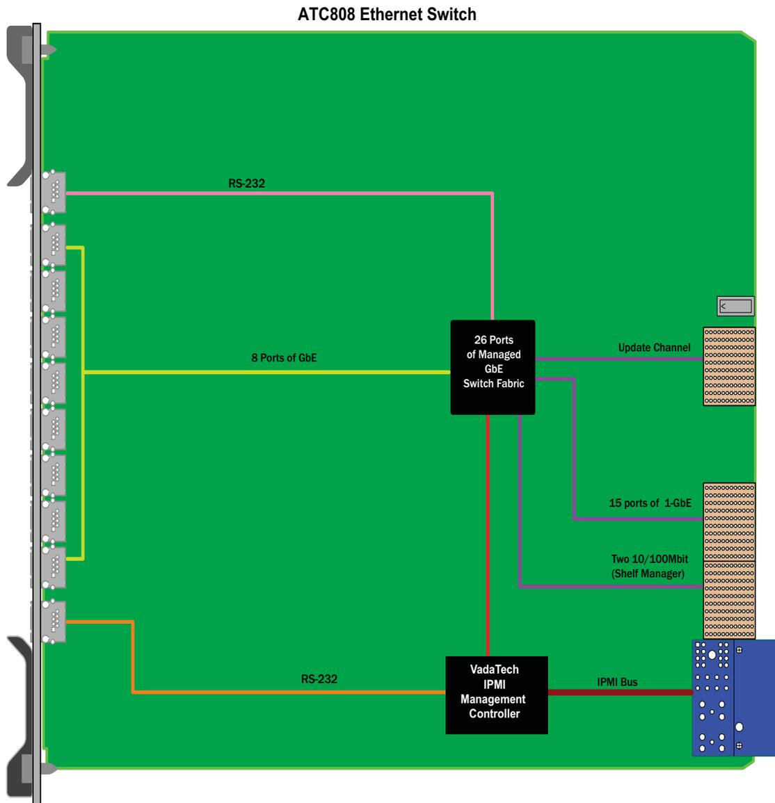
FIGURE 1. ATC808 Functional Block Diagram
