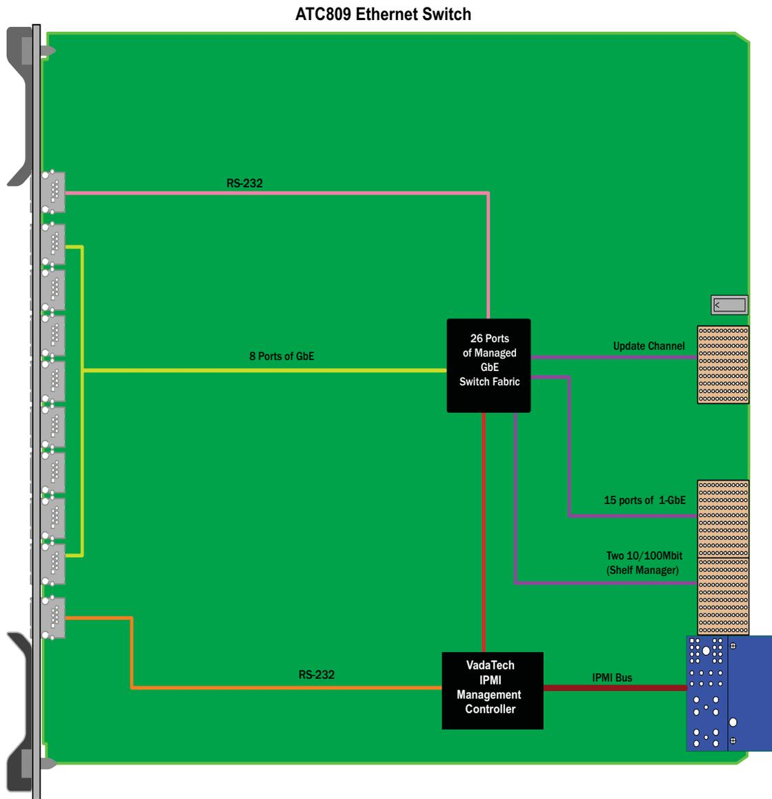
**FIGURE 1.** ATC809 Functional Block Diagram
