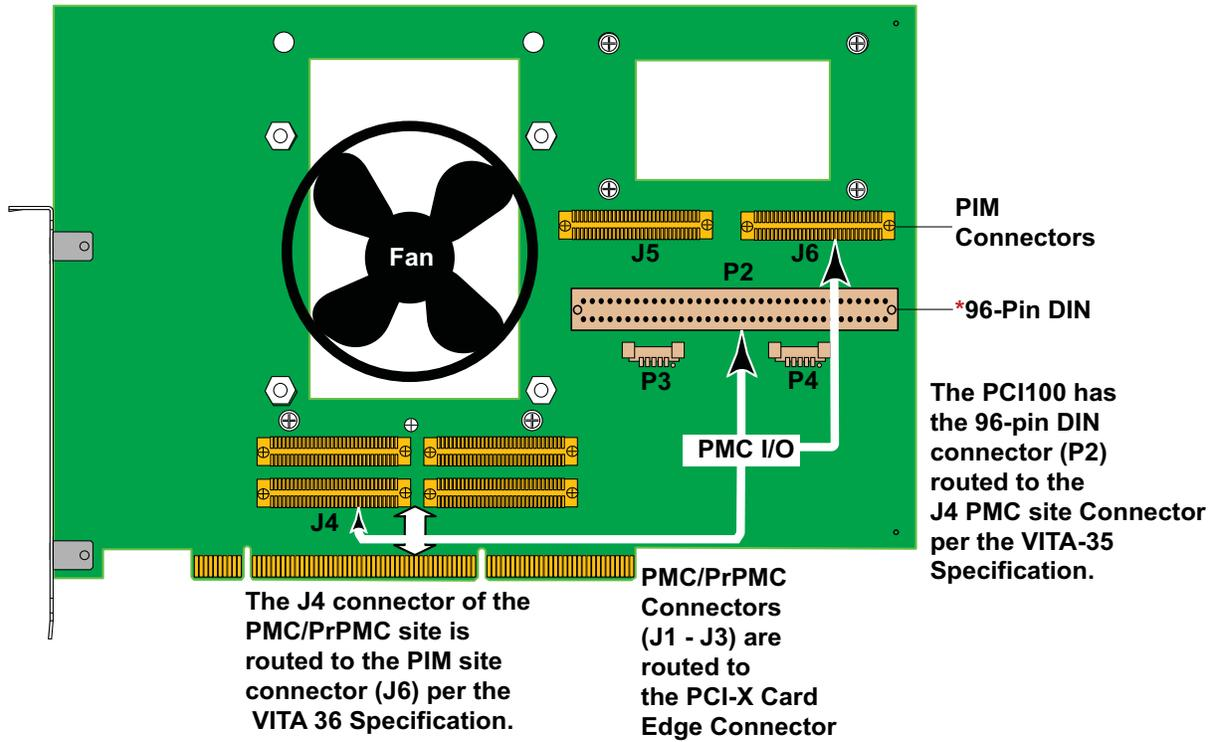
**NOTE:** \*P2 is a 96-pin connector with only 64-pins used.
