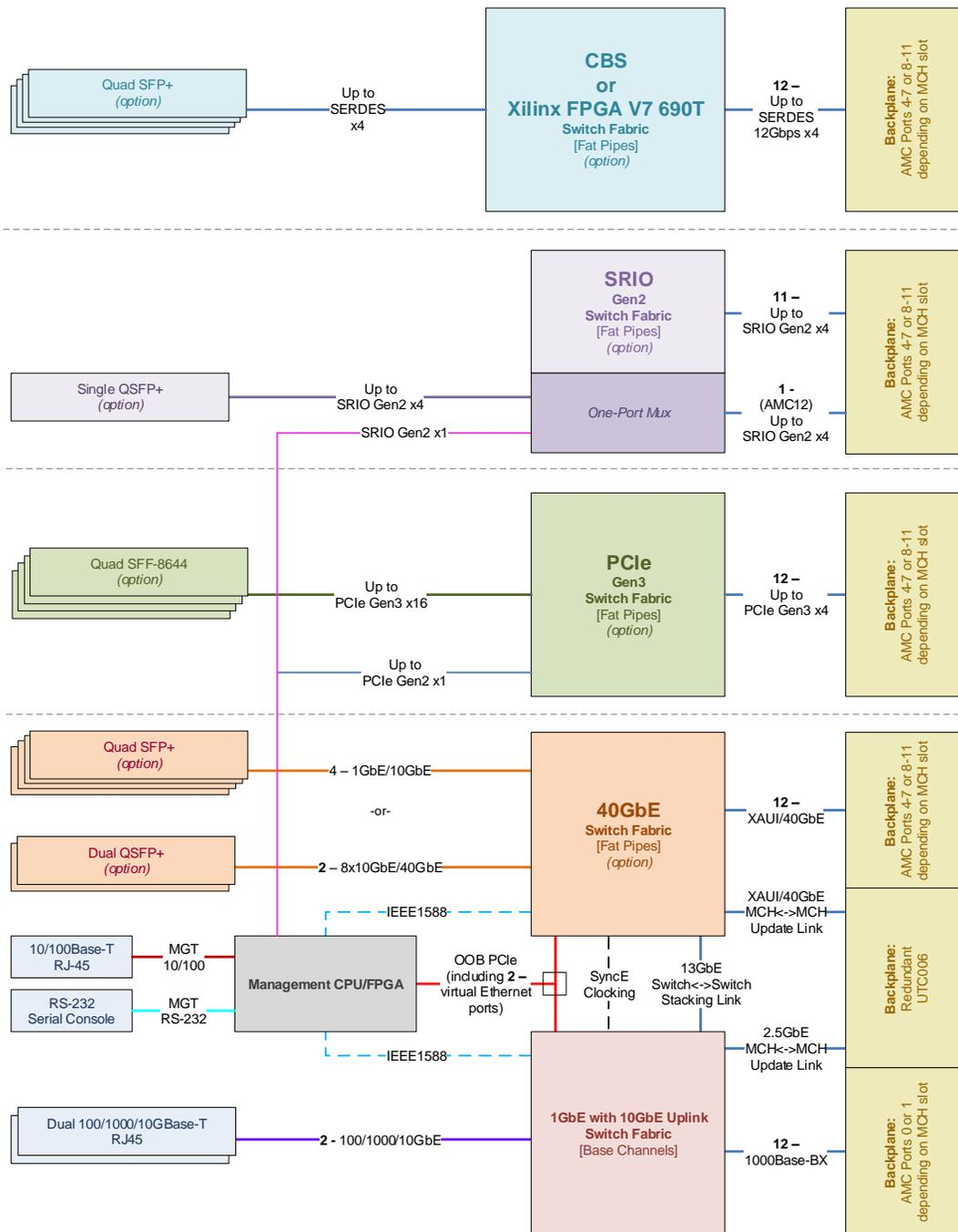
Figure 10: Block Diagram - Connectivity and Fabric Options
