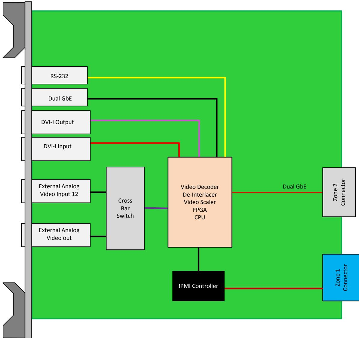
Figure 1: ATC342 Block Diagram
