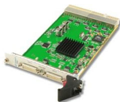
CP341 cPCI Dual Channel DVI/VGA
