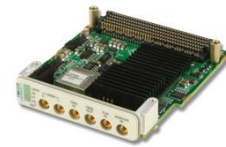
FMC210 ADC 10-bit 2.6 GSPS
