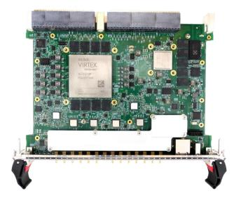
Figure 2: VPX577 without Heatsink
