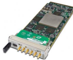
AMC526 AMC Dual ADC, Virtex-7, 12-Bit @ 2.6 GSPS
