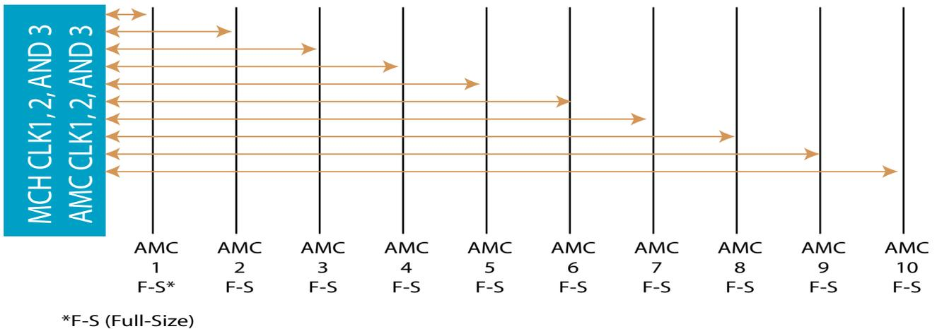
FIGURE 5. VT862 non-redundant clock Topology, CLK3 can run as Fabric Clock (i.e. PCIe clock)
