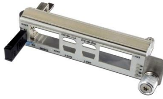
Figure 1: Single Latching Flange Panel Design Example
